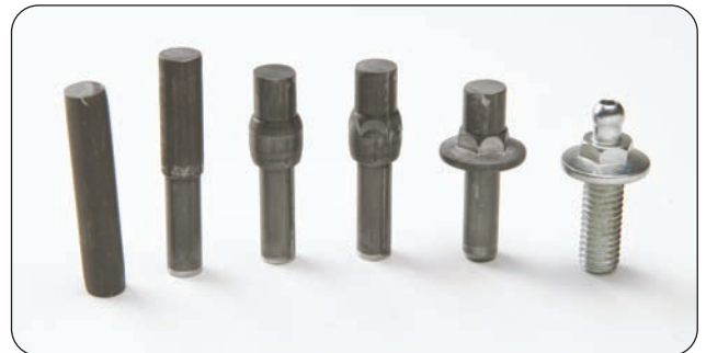
Photo above depicts a cold forming progression. Parts first start as a raw blank and then are progressively formed with dies to shape and trim parts.
